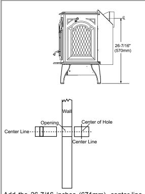
Add the 26-7/16 inches (671mm), center-line measurement to the depth measurement of your floor protector. Mark this <u>combined measurement</u> at the correct wall location for your installation, maintaining minimum clearance to combustibles.
